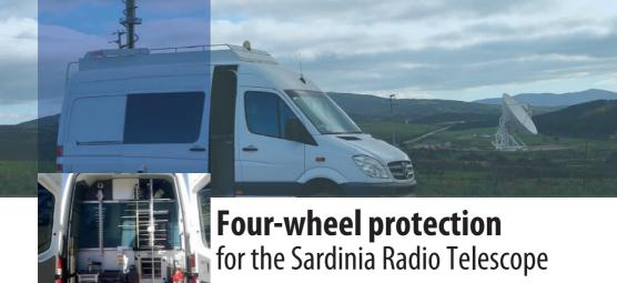
MobLab - Mobile instrumentation for the search for artificial radio interference
