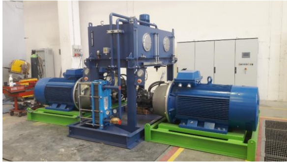
Autofrattage and fatigue test pumping unit for 10000 cycles
