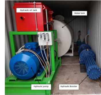
Burst test pumping unit up to 1000 bar
