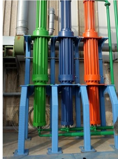
Autofrattage and fatigue test pumping unit for 10000 cycles
